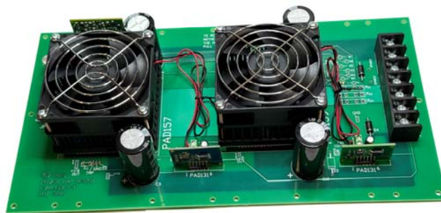
Assembled EVAL159 with PAD157 and PAD159 mounted. Optional PAD125 and PAD131s also shown.
