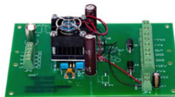
PAD04 MOUNTED IN EVAL04 EVALUATION KIT
