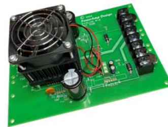
PAD146 mounted in EVAL146 evaluation kit
