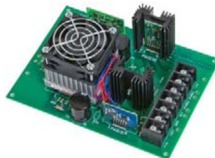
Assembled EVAL129 with amplifier mounted. Optional accessory modules PAD125, PAD132 and PAD131 also shown.
