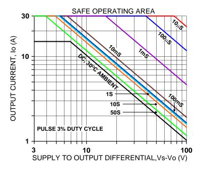
While the graph above adequately shows DC SOA and some pulse information it does not take into account ambient temperatures higher than 30°C, AC sine, phase or non-symmetric conditions that often appear in real-world applications. The **PAD Power** TM spreadsheet takes all of these effects into account.
