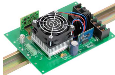
PAD117A mounted in EVAL117 evaluation kit with accessory modules.
