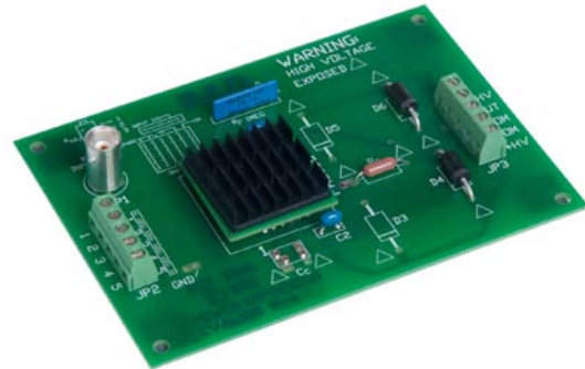
Assembled EVAL188 with amplifier installed.
