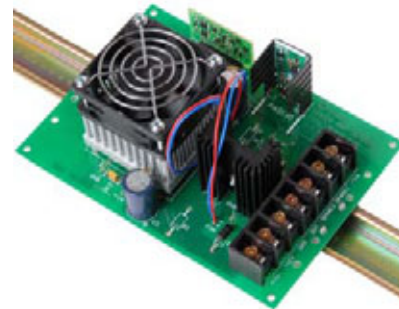
PAD129 mounted in EVAL129 evaluation kit with accessory modules.
