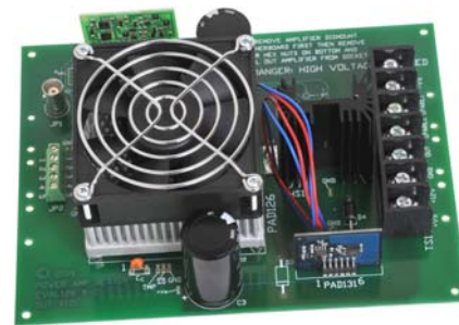
PAD126 MOUNTED IN EVALUATION KIT WITH OPTIONAL ACCESSORY MODULES PAD125 & PAD131
