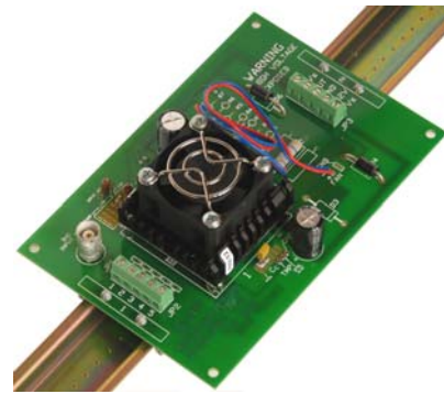
PAD113 INSTALLED IN EVALUATION KIT
