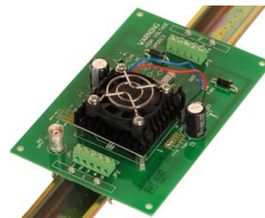
PAD112 INSTALLED IN EVALUATION KIT
