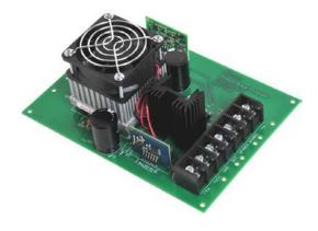
Assembled EVAL137 with amplifier and optional accessory modules installed.
