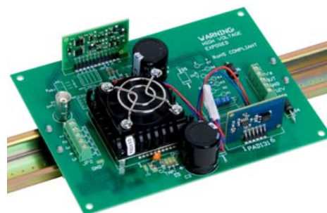
Assembled EVAL112 with amplifier installed. Optional accessory modules also installed. Optional 35mm DIN rail mounting shown.
